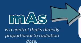
mAs is milliamps seconds. It's going to be directly proportional to the number of electrons that come off of the filament and are accelerated across the gap.
